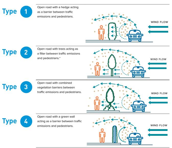
\*Under some conditions, due to a windbreak effect, pollutants can stagnate behind a sparse row of trees, leading to deteriorated downwind air quality (Abhijith and Kumar, 2019).
