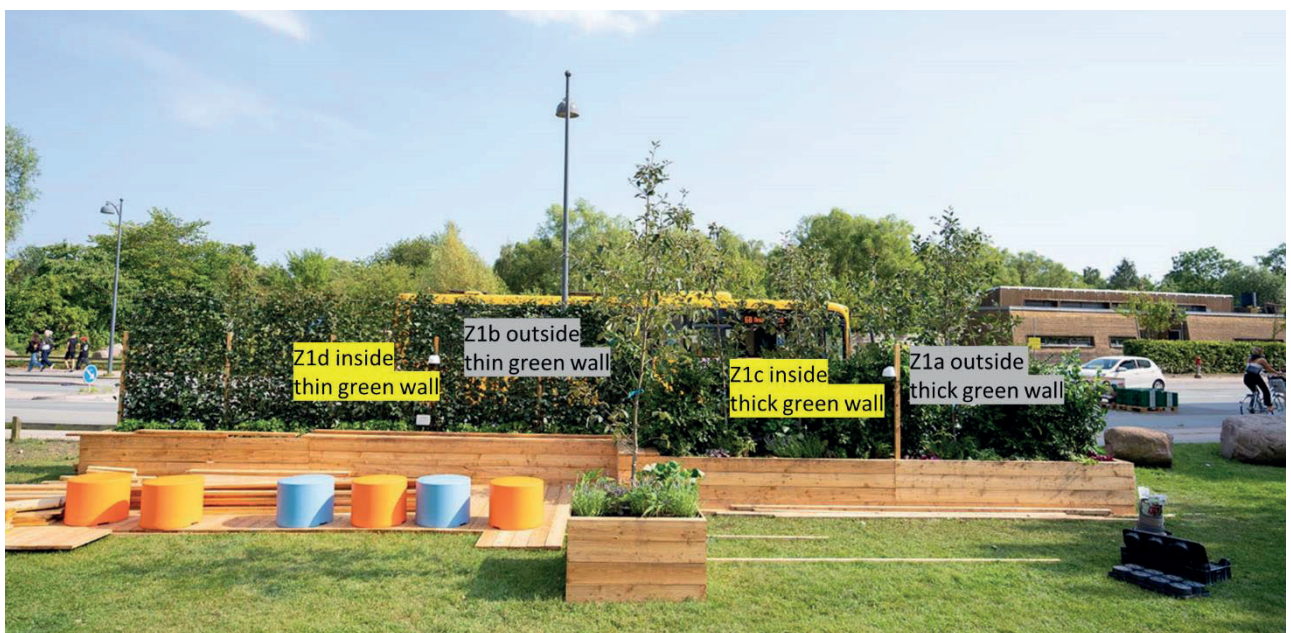
Figure 4: Installation at Havnestaden/Artillerivej site, where the thin green wall is visible on the left side, whereas the thick green wall is visible on the right side.
